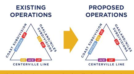
The South Bay Connect route relocation will reduce rail congestion on the Niles and Centerville Line and facilitate the separation of freight and rail services on the busy Niles rail corridor.
